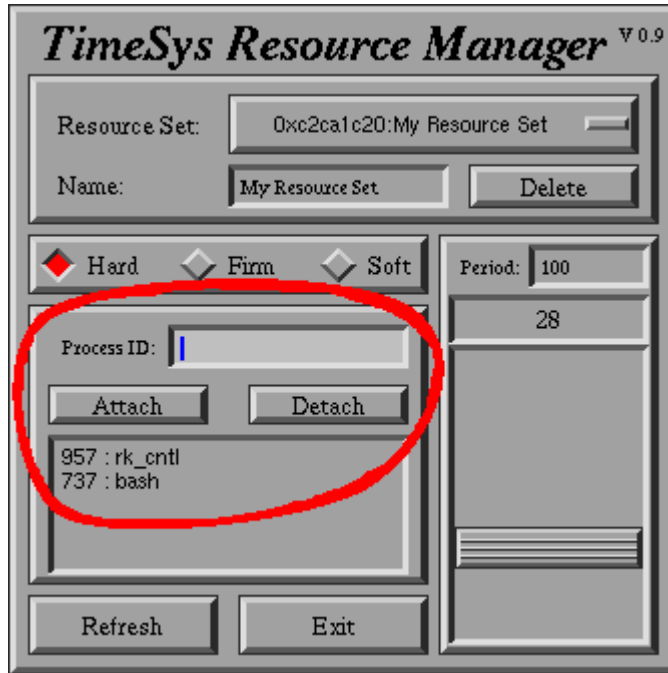
Figure 11: Attaching processes to a resource set
